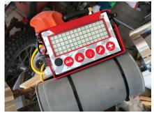
Bring power cable end to the left side of mount. Cut power cable to fit.
